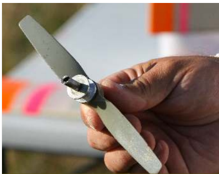
Eliminator eliminated with a broken crank
